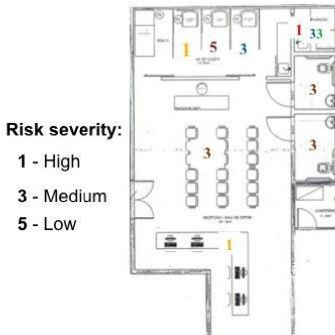
Figure 6. Risk map - Floor plan: numeric indication of severity and the colors of the number indicate risk group
